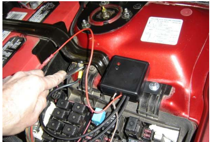
Connect the ground connector to the chassis ground tab.
