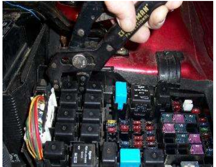
Carefully remove the relays from their sockets.
