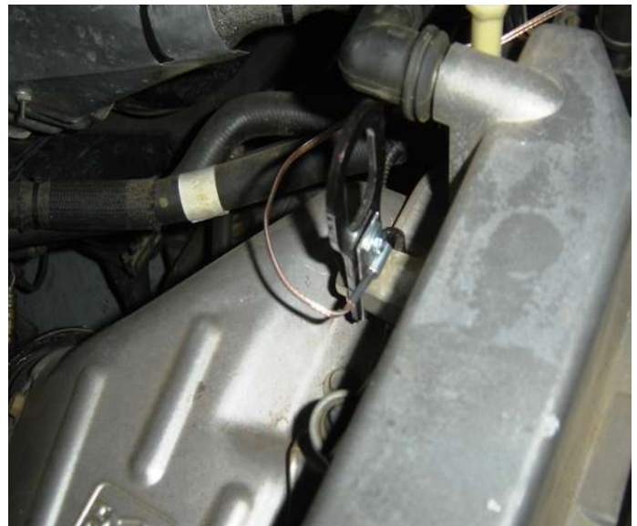
Installation of Block Thermal Sensor on 2.3L I4
