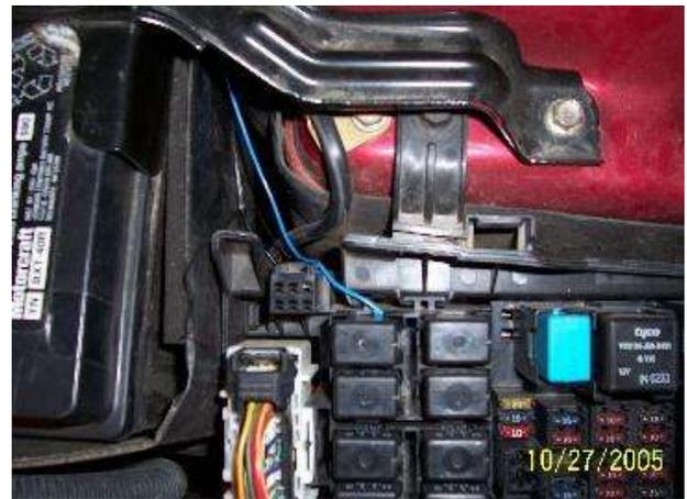
*Replace the fan relay and the relay panel cover.*
