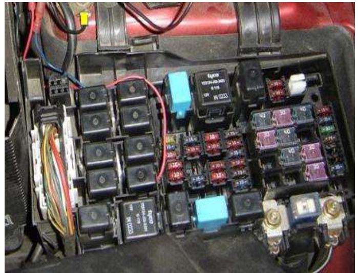
Relays replaced and wires routed to back left corner.
