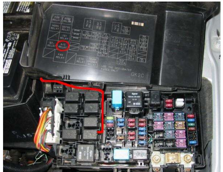
Connect the +12V power lead to the AC Relay
