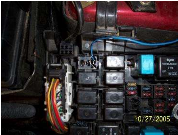
Connect the Blue Fan Relay wire here.
