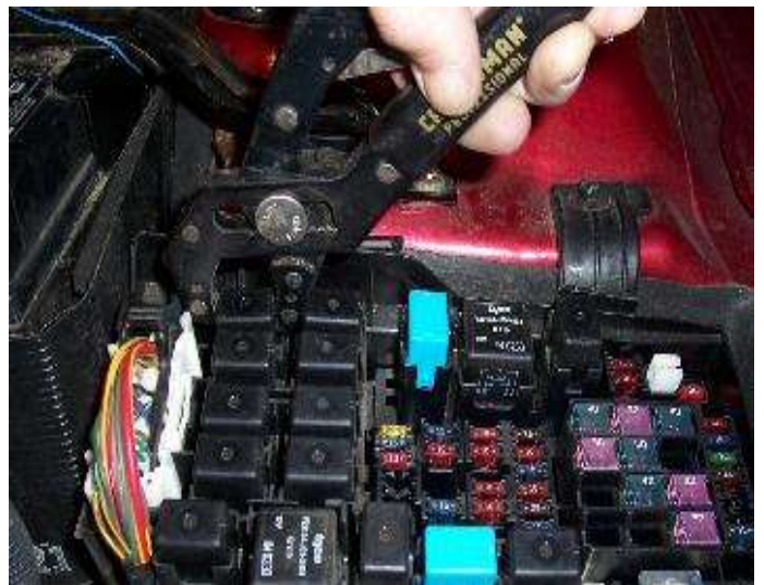
Carefully remove the relays from their sockets.
