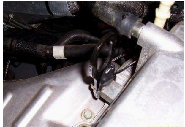
Controller mounted on engine hoist bracket.
