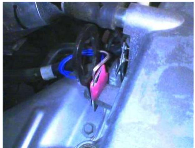
*ATFC mounted on the engine hoist bracket.*
