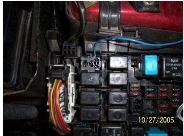
*Connect the controller wire here.*
