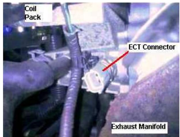
*Close-up of ECT sensor plug on the back of the engine.*
