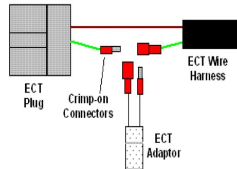
*Connect the ECT Adaptor to the green ECT wires.*
